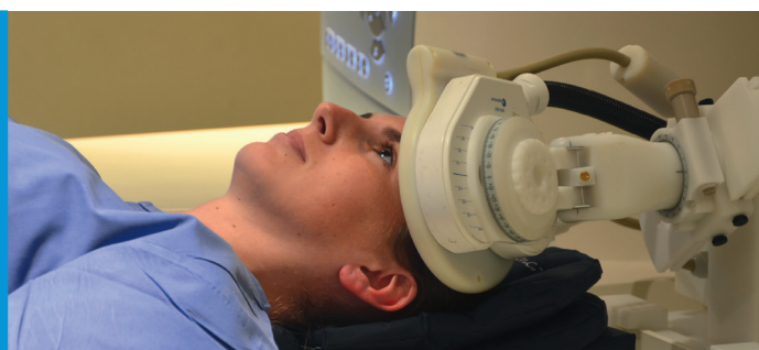
After: The new ultra-thin MR coil array, mounted on the MagVenture MRI B91 Coil.
