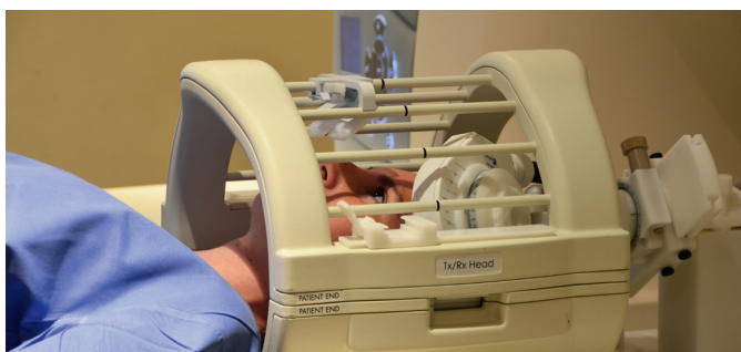
Before: The old standard birdcage MRI head coil.
