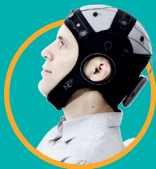
StarStim 8 8 channels, combined tES-EEG, compatible with NIRS
