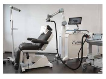
Axilum Robotics Cobot solution ensures movement control and a high level of repeatability and accuracy between TMS sessions. It is especially suited for research and works with MagVenture stimulators and coils. It can be piloted by a neuro navigation system from Localite (MRI guidance).
